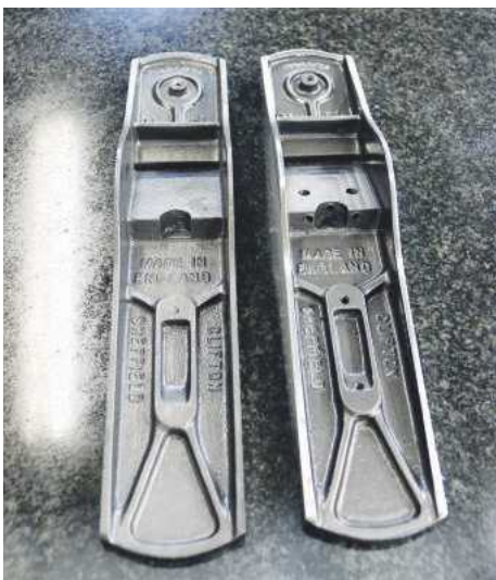
▲ On the right, the finished casting ready to be checked for flatness on the surface plate
